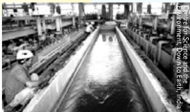
An open mercury-cell at a chlor-alkali plant.
